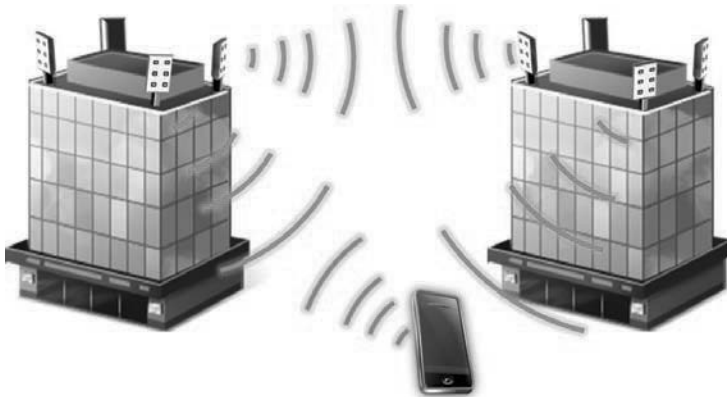
Figure 1.10 Wireless backhaul and relays may be used to connect multiple cell sites and subscribers together, replacing or augmenting copper or fiber backhaul solutions.
