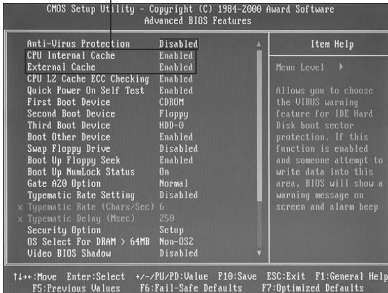
FIGURE 6.22 For accurate results, before testing memory the CPU Internal (L1) and External (L2 and L3) caches should be disabled in the system BIOS Setup on systems having this option.
